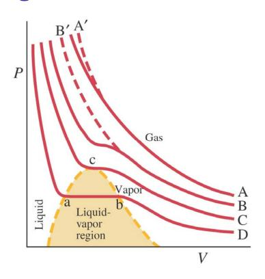
In curve D, the gas becomes liquid; it begins condensing at (b) and is entirely liquid at (a). The point (c) is called the critical point.
