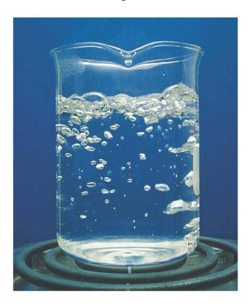
A liquid boils when its saturated vapor pressure equals the external pressure.
