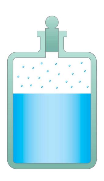
An open container of water can evaporate, rather than boil, away. The fastest molecules are escaping from the water's surface, so evaporation is a cooling process as well.
