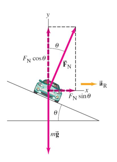
Banking the curve can help keep cars from skidding. When the curve is banked, the centripetal force can be supplied by the horizontal component of the normal force. In fact, for every banked curve, there is one speed at which the entire centripetal force is supplied by the horizontal component of the normal force, and no friction is required.
