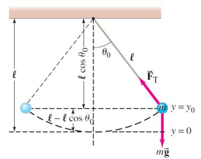
(a) Describe the motion of the bob in terms of kinetic energy and potential energy. Then determine the speed of the bob (b) as a function of position  $\theta$  as it swings back and forth, and (c) at the lowest point of the swing. (d) Find the tension in the cord,  $\vec{\mathbf{F}}_{T}$ . Ignore friction and air resistance.
