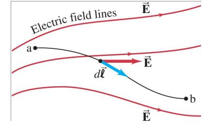
$$V_{\text{ba}} = V_{\text{b}} - V_{\text{a}} = -\int_{\text{a}}^{\text{b}} \vec{\mathbf{E}} \cdot d\vec{\ell}. = -\sum_{a \text{ to } b} \vec{E} \cdot \Delta \vec{l}$$
