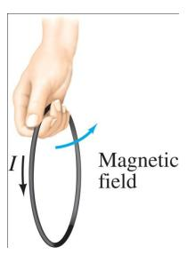
Here we see the field due to a current loop; the direction is again given by a right-hand rule.
