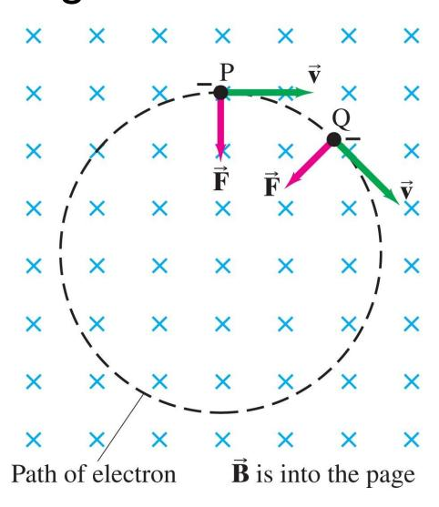
Example 27-7: Electron's path in a uniform magnetic field.
