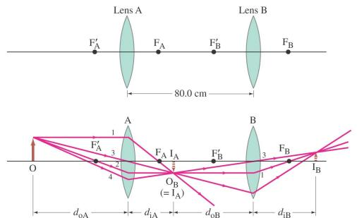
Example 33-6: Measuring f for a diverging lens.
