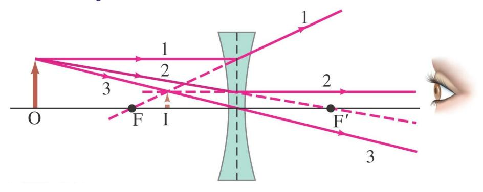
Ray 1 is drawn parallel to the axis, but does not pass through the focal point F' behind the lens. Instead it seems to come from the focal point F in front of the lens. Conceptual Example 33-1: Half-blocked lens.
