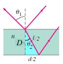
[Solution] (a) We use Snell's law to calculate the refracted angle within the medium. Then using the right triangle formed by the ray within the medium, we can use the trigonometric identities to write equations for the horizontal displacement and path length.
