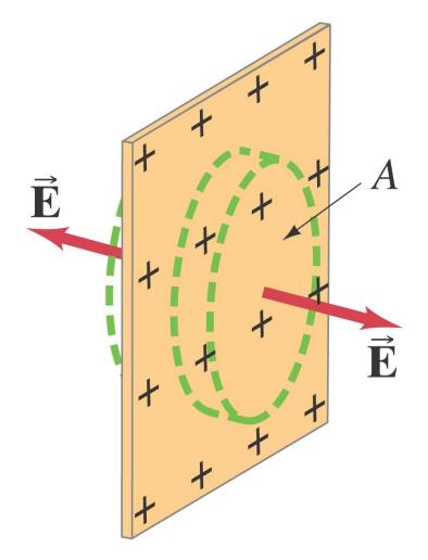
**Example: Electric field near any conducting surface.**
