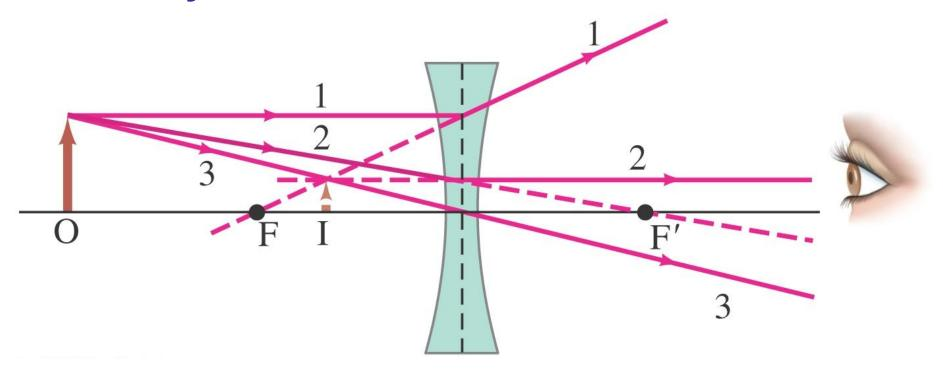
Ray 1 is drawn parallel to the axis, but does not pass through the focal point F' behind the lens. Instead it seems to come from the focal point F in front of the lens. Conceptual Example: Half-blocked lens.
