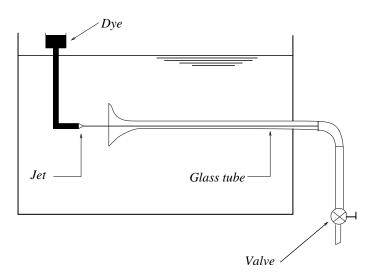
Fig. 4. Reynolds' Apparatus
