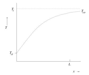
Fig. 6. Temperature Profile of Flow in Tube
