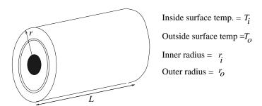
Fig. 3. Hollow Cylinder containing Hot Fluid
