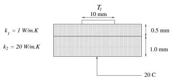
Fig. 2. Circuit Element and its Surroundings
