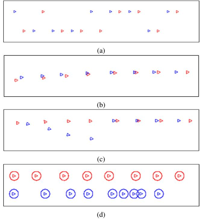
Fig. 9: System snapshots for experiment trial 4: (a) Initial dispersion (b) Convoying manoeuvre makes both red and green choose top lane (c) Robots leaving the devolving lane (d) System achieves maximum speed
