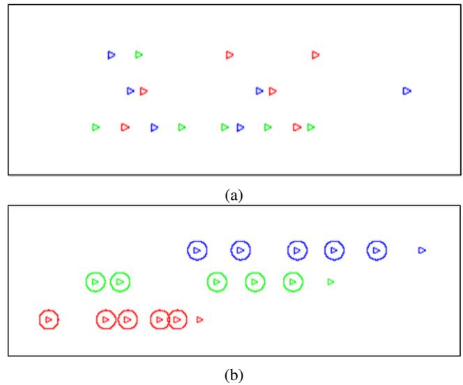
Fig. 10: System snapshots for three categories of robots: (a) Initial dispersion (b) Three lanes formed; one each for a group of like colours
