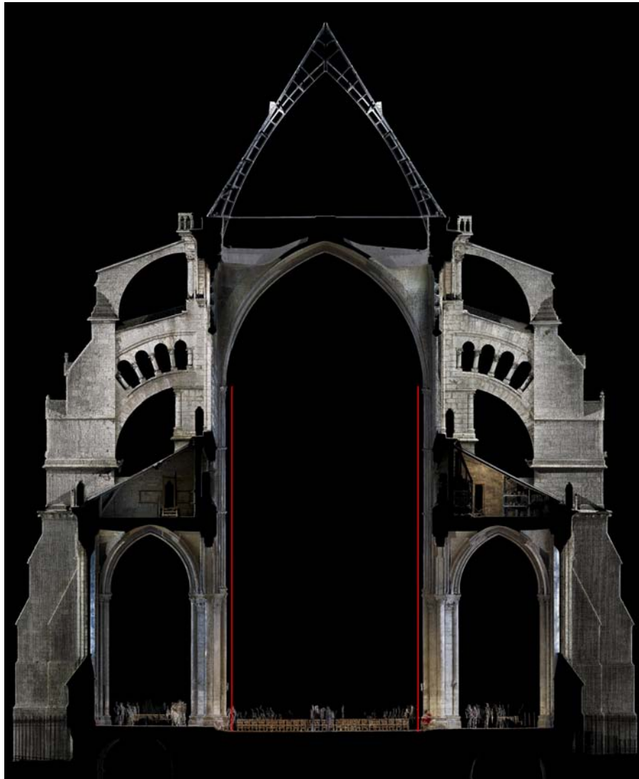
Figure 12 Chartres, Cathedral of Notre-Dame. Section through laser scan data of the nave (image by author)
