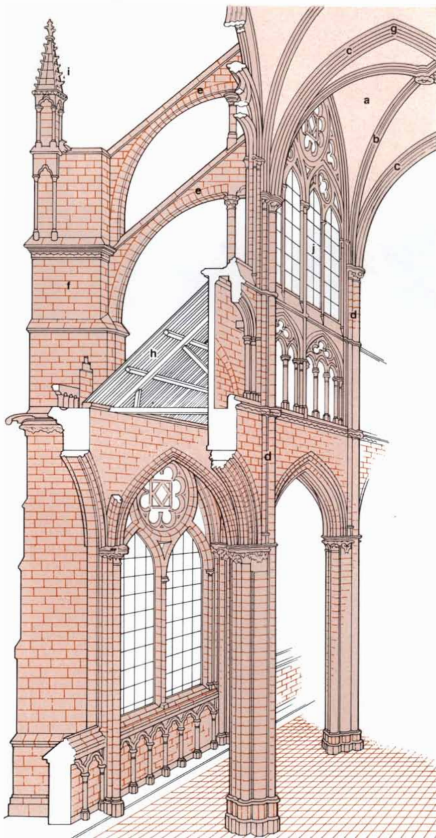
STRUCTURAL CHARACTERISTICS of High Gothic cathedrals are indicated in a drawing of the nave of Amiens Cathedral based on one made by Eugène Viollet-le-Duc. The pointed vaults ( a ) are constructed with a system of diagonal ( b ) and transverse ( c ) ribs on tall piers ( d ). The piers are supported by flying buttresses ( e ) that run to exterior pier buttresses ( f ). Other structural elements are the vault keystone ( g ), the side-aisle roof ( h ) and the pinnacle ( i ). The windowed wall area above the side-aisle roof is the clerestory ( j ).
