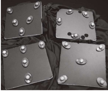
Figure 5. Tags consist of five reflective markers in a configuration that is unique, independent of orientation.
