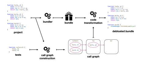
Fig. 6: *Stubbifier* overview with bundler integration. As in Figure 1 a call graph is computed from the project and its test suite, but here the project is bundled before being transformed. The code transformation is applied to the bundle w.r.t. the call graph computed from the application (note: test suites typically rely on the non-bundled application, which is why the call graph is not computed over the bundle directly).
