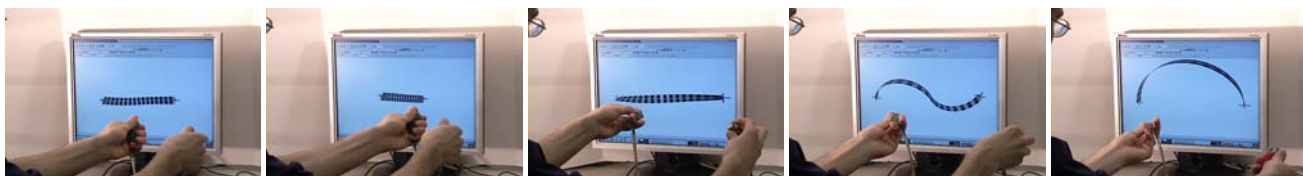
Figure 3: The user manipulates two 6 DOF trackers to control the shape of the ribbon. Note that only the ribbon is shown and no shape is being deformed.
