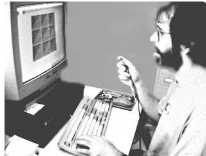
Figure 3: The One-Handed interface. The right hand holds the Bat, and the left hand manipulates the 1, 2, and 3 keys.
