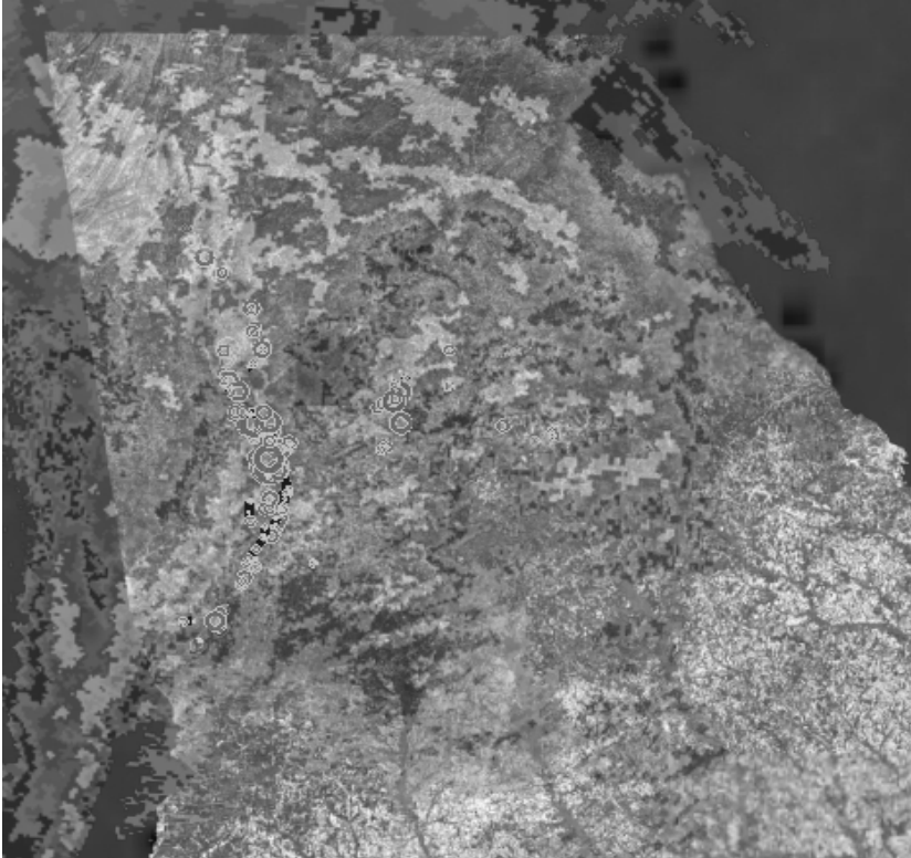
Fig. 3 Interactive view of North Georgia with Doppler radar shown as false-color texture plus mesocyclones shown as semitransparent cylinders.
