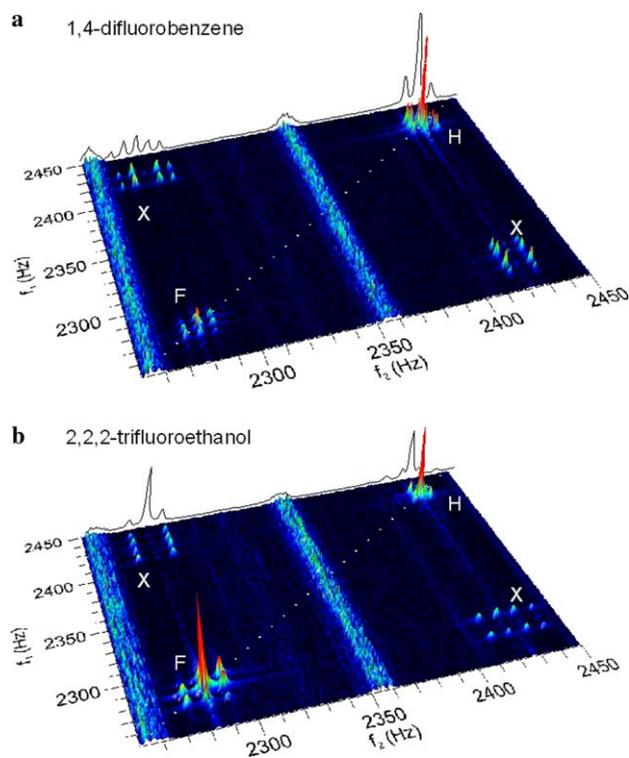
Fig. 2. Experimental 2D COSY NMR spectra for (a) difluorobenzene and (b) trifluoroethanol. Both were obtained at audiofrequencies 2.28 kHz ( $^{19}\text{F}$ ) labelled F, and 2.43 kHz ( $^1\text{H}$ ) labelled H. X represents the cross-peaks). The streaks along  $f_1$  are from low frequency interference.
