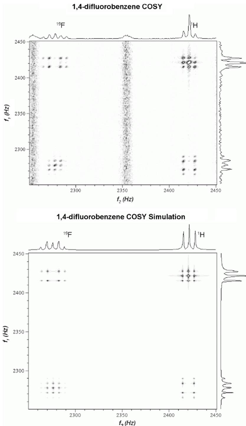
Fig. 3. Experimental and simulated 2D COSY NMR spectra for difluorobenzene shown as contour plots. The projected  $f_1$  and  $f_2$  domain 1-D spectra are shown to the right and above each 2D plot, respectively. The experimental data are equivalent to that shown as a surface plot in Fig. 2.
