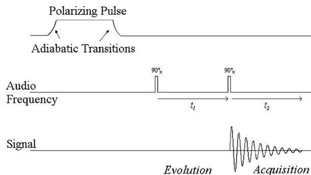
Fig. 1. Timing sequence showing the pre-polarising pulse (duration around 6 s), and the two phase-locked audiofrequency excitation pulses. The evolution period is  $t_1$  and the acquisition time domain is  $t_2$ .
