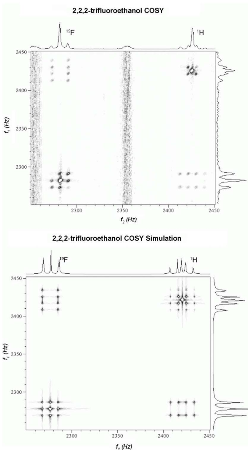
Fig. 4. Experimental and simulated 2D COSY NMR spectra for trifluoroethanol shown as contour plots. The projected  $f_1$  and  $f_2$  domain 1-D spectra are shown to the right and above each 2D plot, respectively. The experimental data are equivalent to that shown as a surface plot in Fig. 2.
