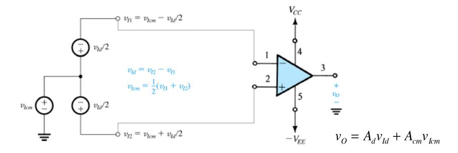
Common-Mode Rejection Ratio (CMRR) quantifies the op amp's ability to reject the common mode signals
