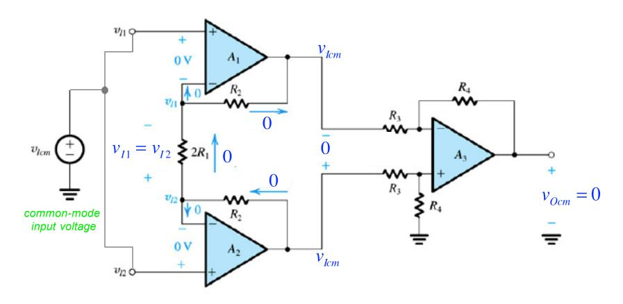
The input stage  $A_1$ ,  $A_2$  no longer amplifies the common-mode signal; it simply propagates it to the  $A_3$  input, where it becomes supressed by  $A_3$ .
