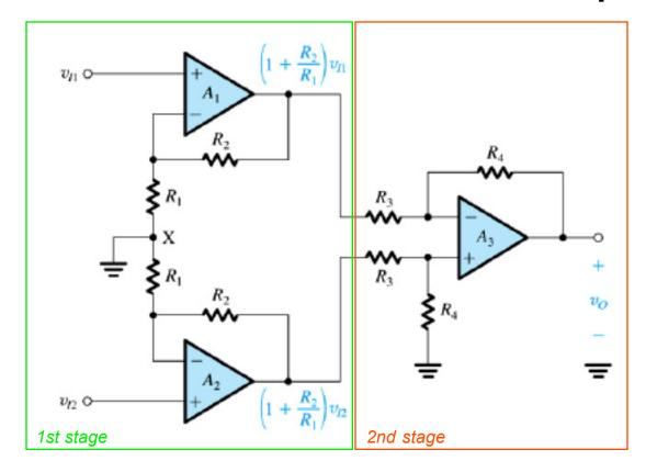
1st stage - noninverting op amps A<sub>1</sub> and A<sub>2</sub> to increase the input resistance
