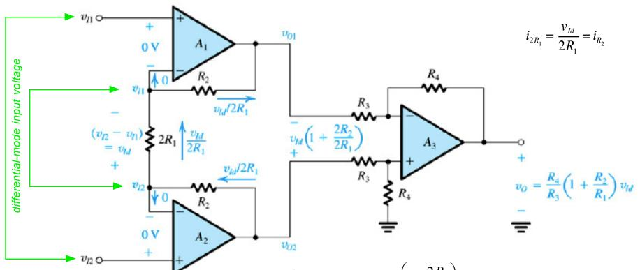
$$v_{O2} - v_{O1} = \frac{v_{Id}}{2R_1} (2R_1 + 2R_2) = v_{Id} \left(1 + \frac{2R_2}{2R_1}\right)$$
