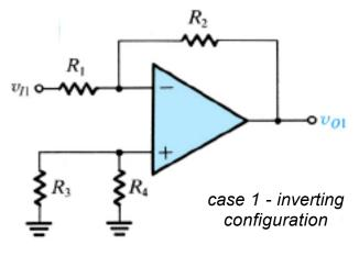
$$\frac{R_4}{R_3} = \frac{R_2}{R_1}$$
