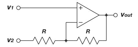
T.2.5 Find an expression for  $v_{out}$  as a function of  $v_1$  and  $v_2$  in the op amp circuit shown below, and determine the input resistances seen by each input in this configuration. Assume that op amps are ideal.
