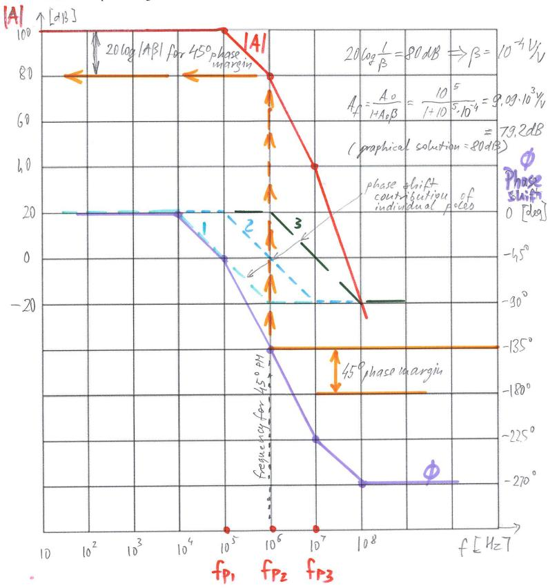
Consider a feedback amplifier for which the open-loop gain A(s) is given by:
