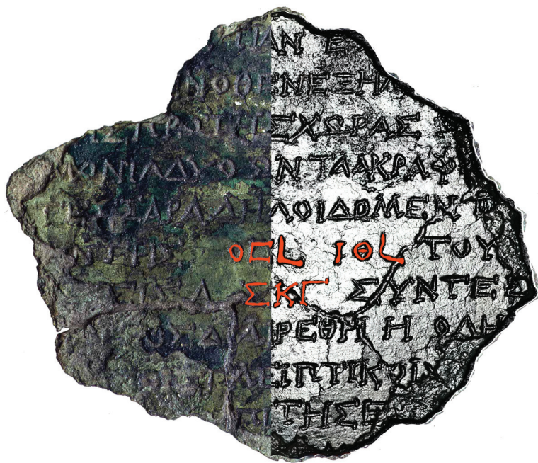
Figure 1. Applying surface imaging to fragment 19, the Antikythera mechanism's back cover: (left) photograph and (right) reflectance transformation image that enhances the text in what amounts to the mechanism's instruction manual. The text highlighted in red identifies the ancient Babylonian cycles that underlie the gearing: "76 years" refers to the Callippic cycle, "19 years" to the Metonic cycle, and "223" to the Saros cycle. Copyright 2006-2008 Antikythera Mechanism Research Project.
