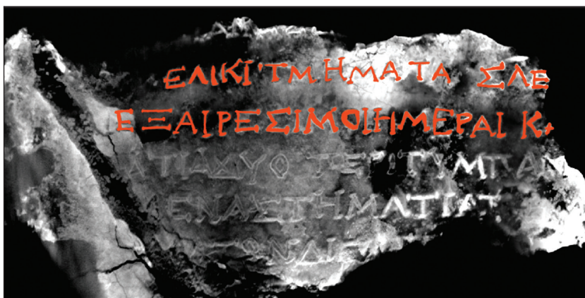
Figure 3. Composite of several X-ray CT slices through Fragment E, which form part of the back cover. The text is roughly 1.6 mm high, and the only word visible on the surface is EAIKI, meaning "spiral." The highlighted text reads "Spiral subdivisions 235" and "Excluded days twenty [two]." These both refer to the mathematical organization of the 19-year Metonic calendar dial. Copyright 2006-2008 Antikythera Mechanism Research Project.
