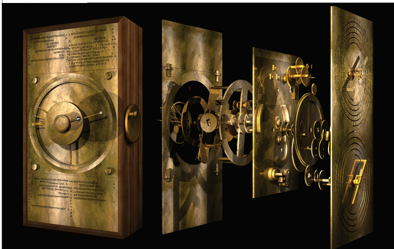
Figure 5. Computer reconstructions using Lightwave 3D. (left) The mechanism's front, showing pointers for the date, sun, moon, and three conjectural planets: Mercury, Venus, and Mars. The inscriptions are a calendar describing the rising and setting of stars in the annual cycle. (right) Exploded model, showing the complexity of the lunar anomaly mechanism's gearing as well as sliding pointers that follow the spiral dials of the Metonic calendar and the Saros eclipse prediction scale. Copyright 2011 Images First Ltd.
