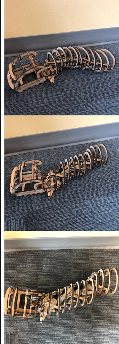
Category 03 ABM - the mechanical parts are the machine. No extra part is added without a mechanical function/output; except the arches repeated to represent insect's body perhaps. The mechanical parts move in a motion inspired by a slithering snake-like insect.
