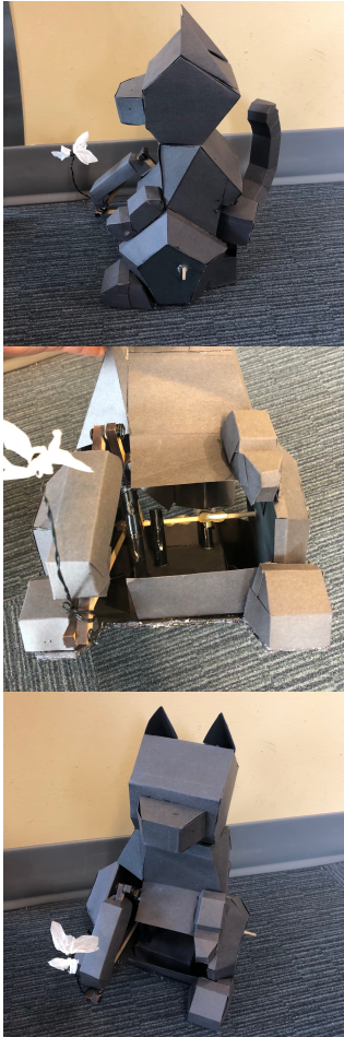
Category 01 ABM - housing holds the mechanical parts (Housing is made out of paper, folded and glued to achieve origami effects)
