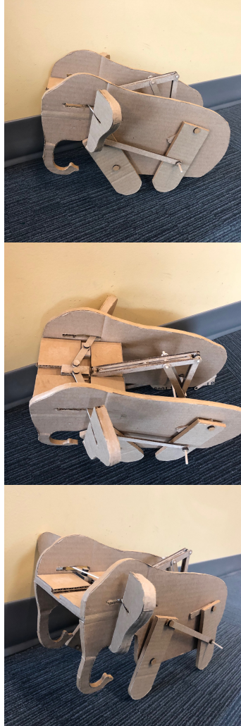
Category 02 ABM - the mechanical parts integrate with the housing to create the overall effect. In this case the linkage mechanism is used outside the elephant's body to represent its legs creating a beautiful walking motion.
