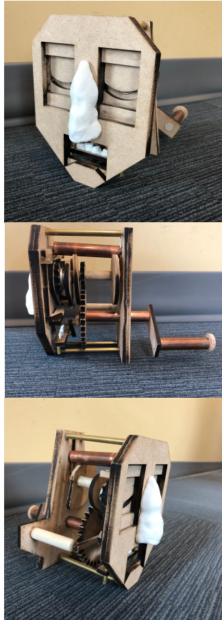
Category 02 ABM - the mechanical parts integrate with the housing to create the overall effect. In this case the skull and the complexity of ideas in one's head are depicted using complex chains of gears, cams and linkages.
