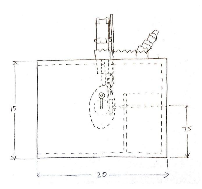
This Right view shows details of the "front-back" spacing, for main axle, 3bar support partition, and croc jaw location.
