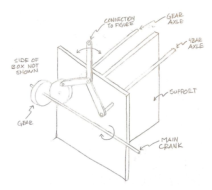
Here we see a first cut at showing not only the mechanism for moving the monkey, but the necessary support structure.
