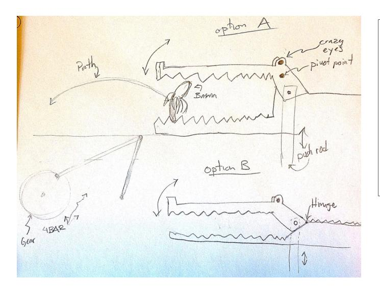
Here, options for the croc are explored in a bit more detail, and the path is shown with respect to the croc's mouth.
