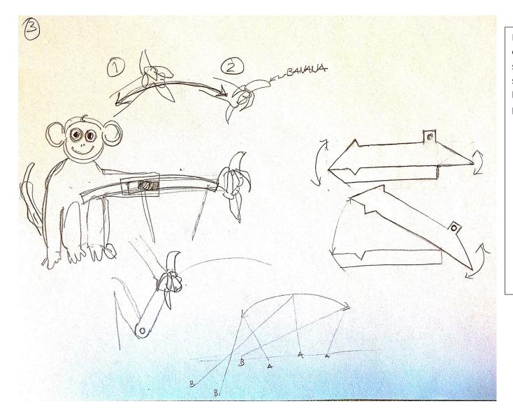
Here more detail is set out, based on the previous sketches. The 4-bar is sketched in 3 positions, both extremes and a mid position.
