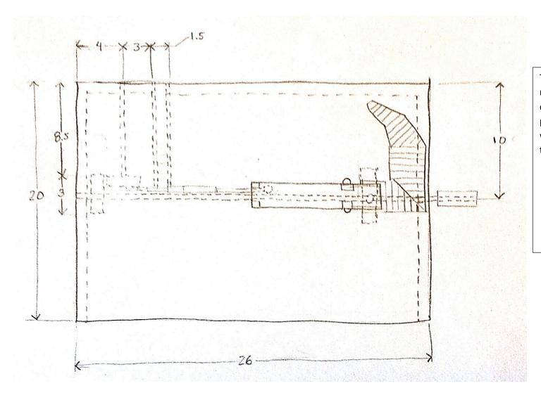
The last ortho view is needed to specify details of axle and partition locations, as well as the location of the croc and tail.
