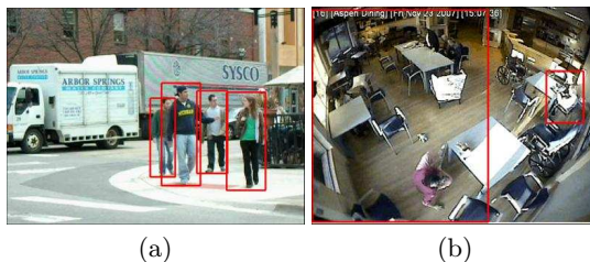
Fig. 5. Typical results of running a state-of-the-art pedestrian detector [12] on the two datasets used in the experiments. On the collective activity dataset (a), the detector performs very well. But on the more challenging nursing home dataset (b), the detector is not reliable since the videos are captured by a fish eye camera, so persons in the videos are not in upright positions. In addition, the video quality is very poor.
