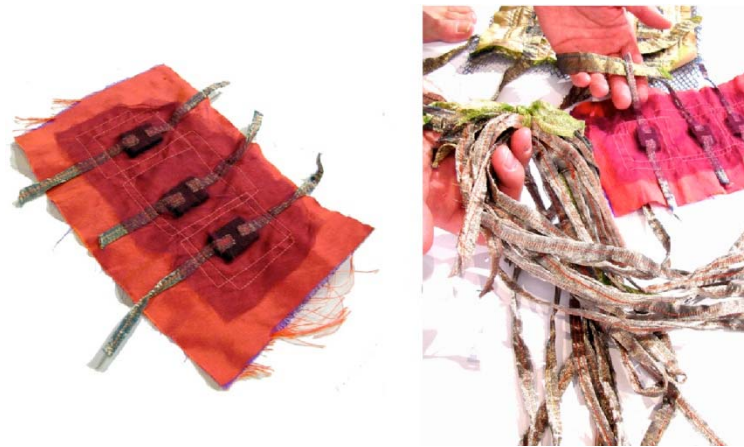
Figure 80. Touchpad with Conductive Foam as Taxel and Conductive Fabric as Wire (2005)
