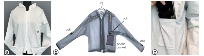
Figure 10: Proof-of-concept NFCe jacket: (a) results; (b) locations of the relays; (c) phone pocket.
