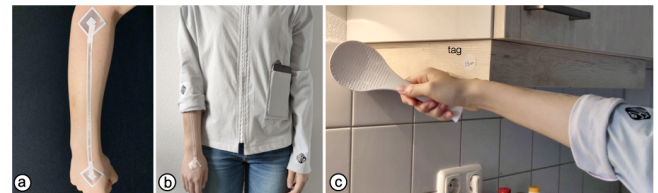
Figure 14: The elbow coil on the jacket is extended by an on-body relay sticker so the user can use her wrist to access a personal shortcut.
