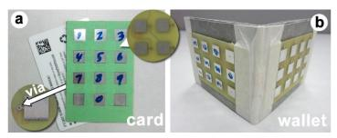
**Fig. 2.** Left: Card-shaped CipherCard with a 3×4 electrode grid. Top callout shows the internal wiring and bottom callout shows the via and electrodes on the back. Right: Wallet-based CipherCard.
