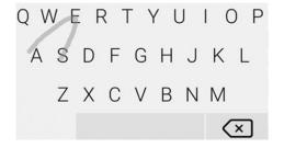
Figure 4: The gesture trajectory of the word "sea" passes the keys "s". "e", "w", and "a" so our system converts the x,y representation of the trajectory into a series of "s", followed by a series of "e", a series of "w", and then a series of "a".
