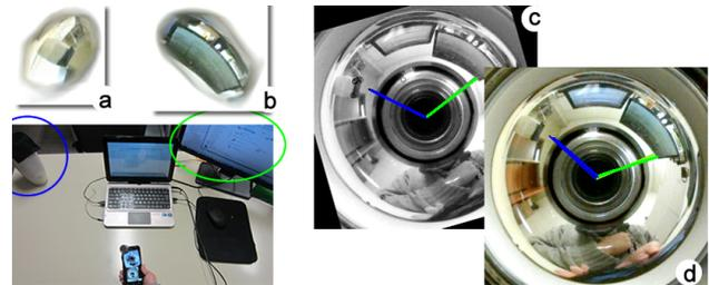
**Figure 3 - Reference images: (a) speaker and (b) monitor; (c) rotated input frame for more precise object detection; (d) recognized objects (the blue and green lines indicate the locations of the recognized objects – speaker and monitor).**
