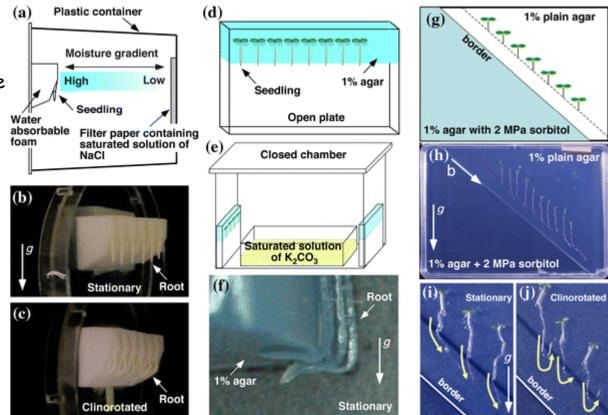
This apparatus can be placed in a clinostat to reduce the effects of gravity.
