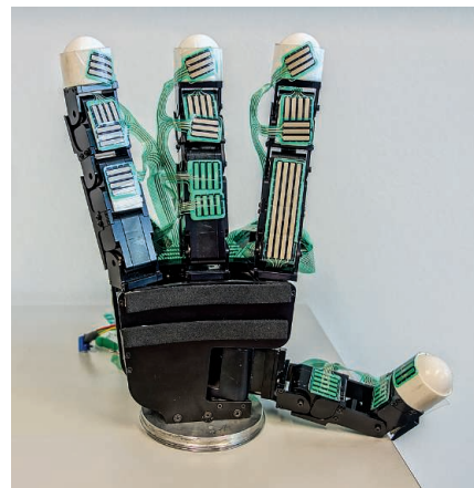
Strategically placed tactile sensors help a robotic hand grasp unknown objects while maintaining low contact forces.
