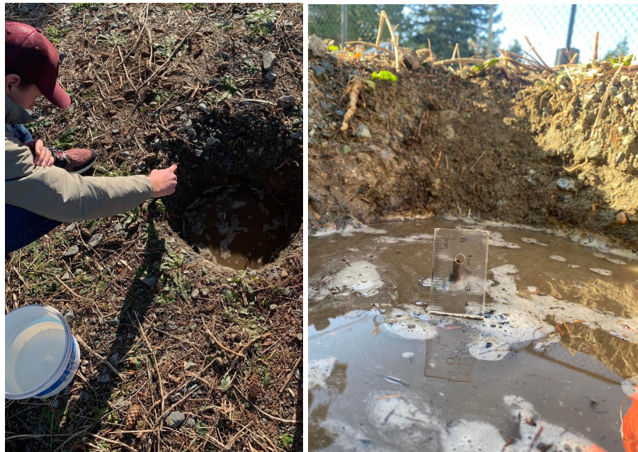
Figure 1: Onsite Infiltration Testing
