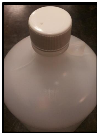
Figure 2. Aqueous waste container with vented cap
