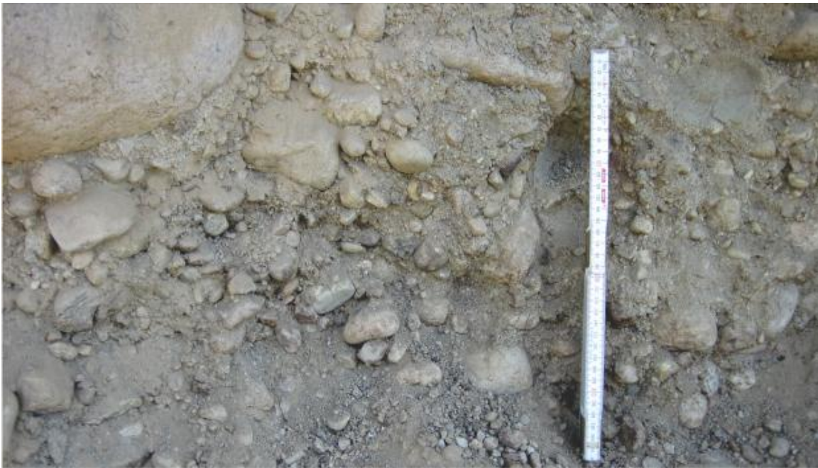
Figure 5-40: Crudely-bedded, clast-supported, massive gravel in a poorly-sorted silty sand matrix with areas of openwork structure exposed at site 48A. Ruler is 0.36 m long.
