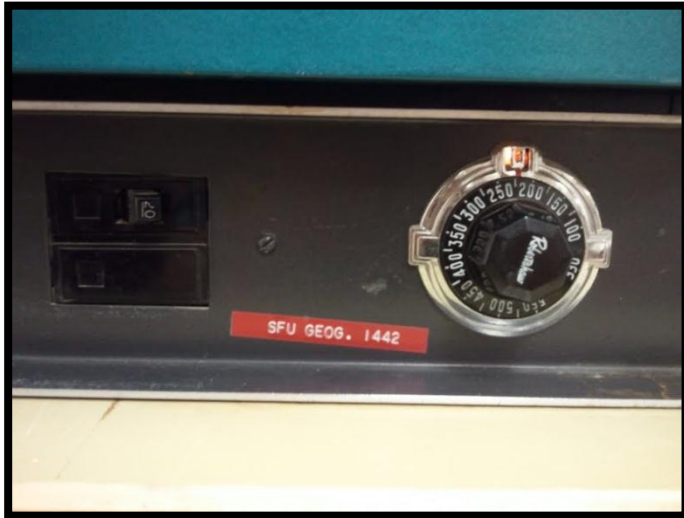
Figure 3. Oven located in RCB6301 where oven drying is performed. The switch (top black bar) in the picture is located in the on position, and the dial is set to 105°C (221°F).
