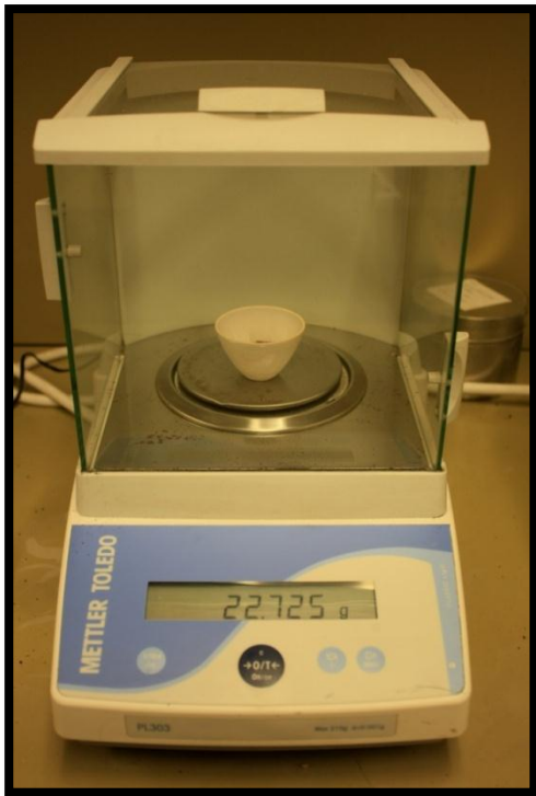
Figure 2. Picture of a scale used to measure the weight of a crucible and sample to 3 decimal places.
