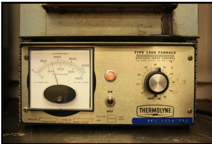
Figure 5. Picture of the oven located in RCB6303. This picture indicates approximately where the knob should be placed during LOI and a suitable temperature reading ( 400^{\circ}\text{C} ).
