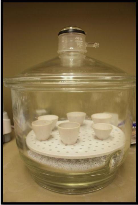
Figure 6. Picture of a desiccator sealed with crucibles in it.
