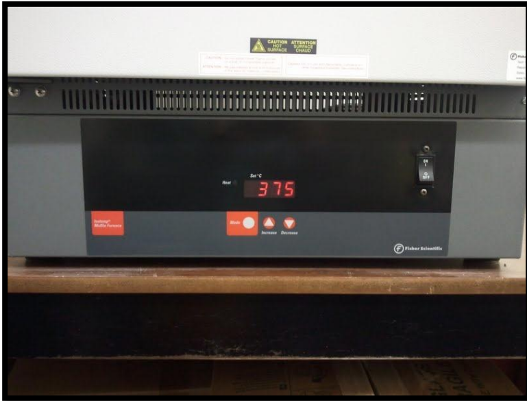
Figure 4. Picture of the muffle furnace located in B6223. The on off switch is located on the front-right, it is currently in the on position. Below the temperature readout are the buttons Mode (used to set the temperature) and Increase and Decrease (used to change the temperature).
