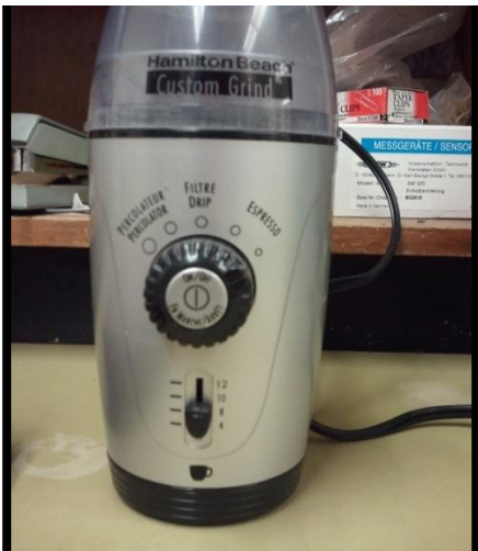
Figure 7. Coffee grinder used to grind forest floor samples. Dial is currently set to espresso, and the ON button is located in the middle of the dial.
