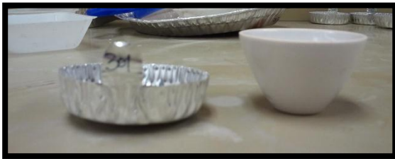
Figure 1. A small metal tin is located on the left, and a crucible is located on the right.
