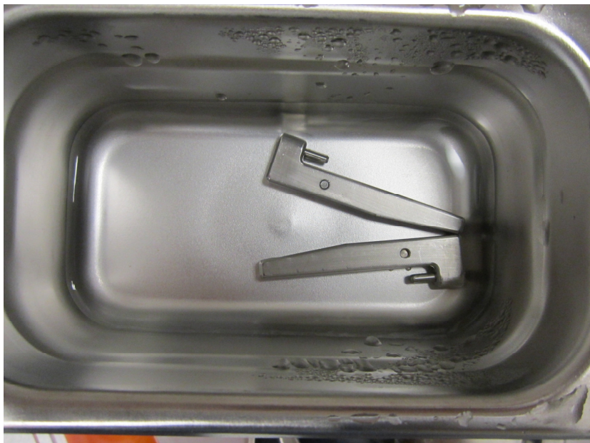
Figure 3. The charge plates in the sonicator.
