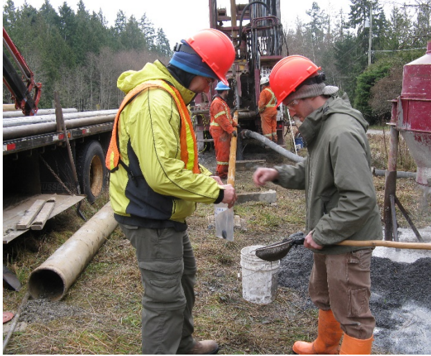
Figure 3. Photograph of collection of rock chips during drilling
