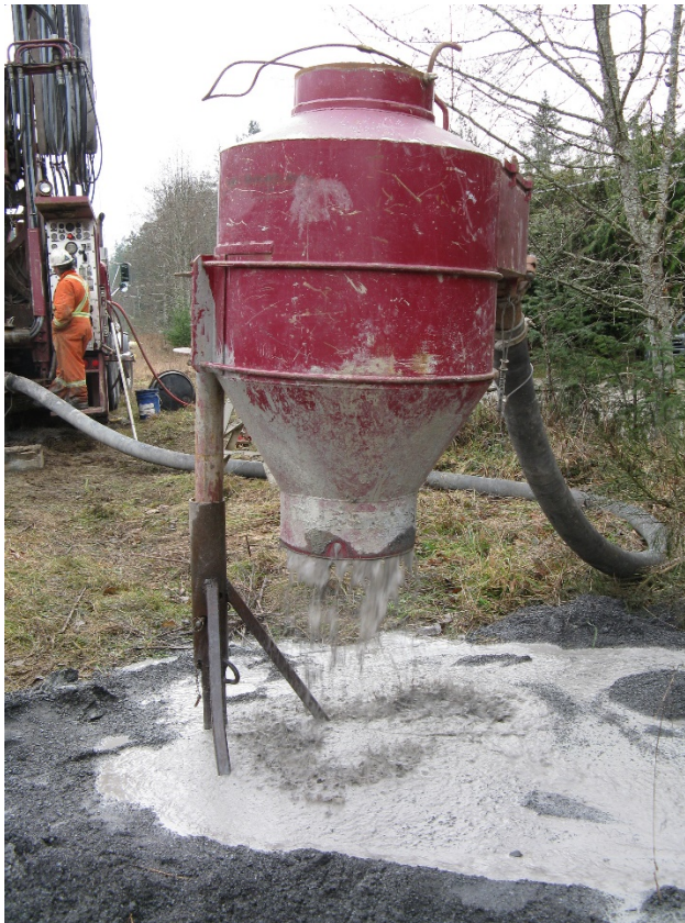
Figure 5. Cyclone employed during drilling.
