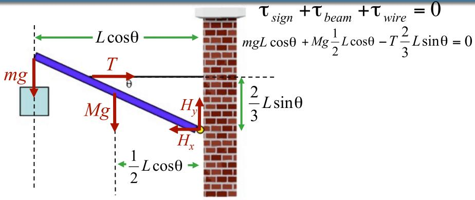
A purple beam is hinged to a wall to hold up a blue sign. The beam has a mass of  $m_b$  = 6 kg and the sign has a mass of  $m_s$  = 17 kg. The length of the beam is L = 2.81 m. The sign is attached at the very end of the beam, but the horizontal wire holding up the beam is attached 2/3 of the way to the end of the beam. The angle the wire makes with the beam is  $\theta$  = 34.1°.
