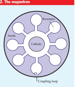
Figure 2. Schematic diagram of a magnetron.
