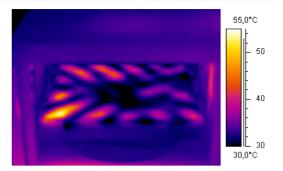
**Figure 4.** Visualization of the horizontal mode structure in a microwave oven using infrared thermal imaging. A glass plate with a thin water film was placed at a height of 8 cm and heated for 15 s with a microwave power of 800 W without using the turntable (for more details on the experiment, see [10]).
