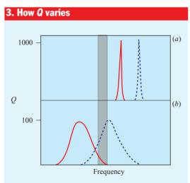
Figure 3. Schematic diagram showing how Q varies with frequency for two different modes of resonance in a microwave oven (not to scale): (a) with oven empty, (b) with food. The shaded band shows the frequency of the magnetron. If drawn to scale the widths of the modes in (b) would be about 100 times those in (a).
