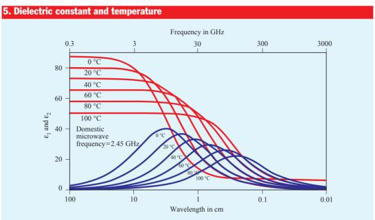
Figure 5. Real and imaginary parts of the dielectric constant  $\varepsilon(\omega)$  for microwaves and various temperatures between 0 °C and 100 °C (after [12]).
