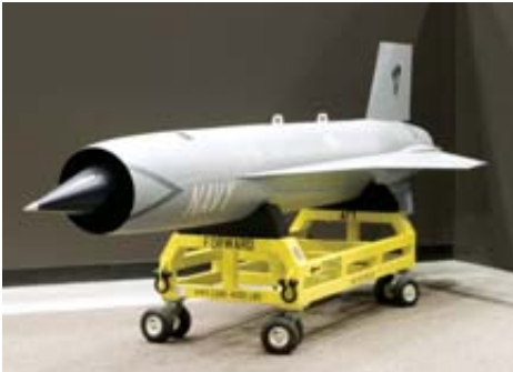
FAST AND FURIOUS: RATTLRS cruise missile, as shown in this mock-up, could set speed records, thanks to a movable air-inlet spike and a novel engine.
