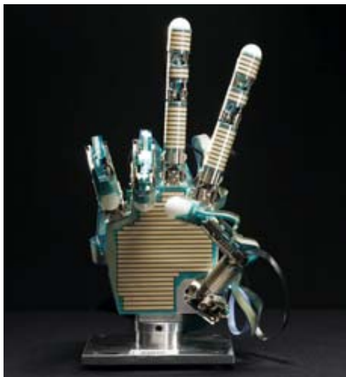
NOT A PEACE SIGN: A mechanical robot hand can form a rock, paper or scissors after being fed data from a player's brain as "read" by an fMRI machine.
