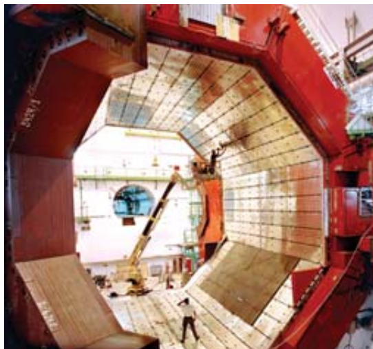
BANG-UP RESEARCH: ALICE detector slated to operate at CERN in 2008 will analyze lead nuclei collisions occurring at about 50 times the energy of RHIC's mini big bangs.
