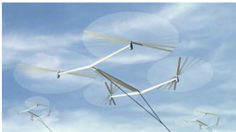
▲ Autogiros designed by Sky WindPower would use powered counterrotating blades to rise above 10,000 feet, then switch to generating mode. Computers adjust the pitch of the four blades to maintain the craft's position and attitude.
