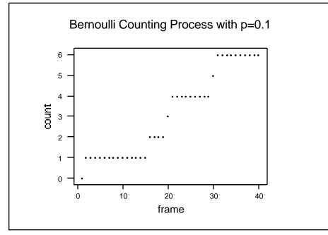
In what frames did "events" occur? How many frames does it take for a change in X(n)? The number of frames from one event to the next event has a geometric distribution and this explains Theorem 7.1-3, p 274.
