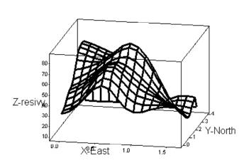
The data portrayed here is taken from a data set of 1000 soil resistivity measurements over a rectangular agricultural area, taken from Cleveland(1993).
