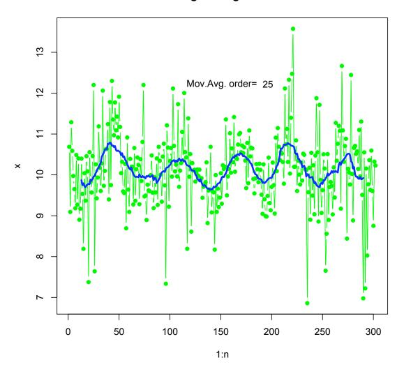
So even the simple moving average (order 25 here) produces the regular sinusoidal pattern in phase with the annual season. With this large data set, the loss of the end points did not matter much (sometimes a problem with the moving average smoothing method.)
