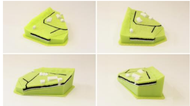
Figure 20: Using more indentation, our system can account for accumulated imprecision of stencil layers.
