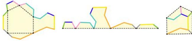
Fig. 6. The boundary of a reversible shape can be divided into congruent segment pairs. Two congruent segments are in the same color.
