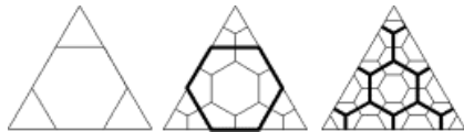
Figure 35: 1-to-3 hexagonal refinement applied to a triangle, as used to generate the ISEA3H. Image taken from [14].
