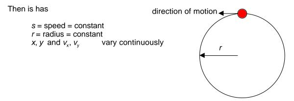
Since s and r are constant, independent of the object's position, they do not specify the position or the velocity the object. While x, y and  $v_x$  and  $v_y$  do describe the object's motion, they are time-dependent and cumbersome.
