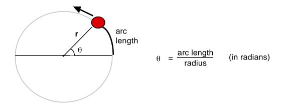
The sign convention is that  $\theta$  increases in a **counter-clockwise** direction. As a function of time,  $\theta$  looks like (for uniform circular motion):
