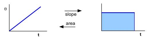
We can go back and forth from  $\theta$  to  $\omega$  by slopes and areas, just like with x and v. For example, from the area under the  $\omega$  vs. t curve, we find
