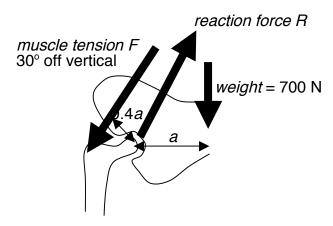
The body weight, acting through its centre of mass, is 700 N and is a perpendicular distance a from the top of the femur. Counteracting this weight is a tension F in a group of muscles running from the femur to the pelvis; we'll represent this as a single force oriented 30° with respect to the vertical, a distance 0.4a from the femur.
