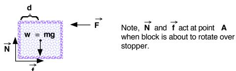
We can use the linear conditions  $\Sigma_i \mathbf{f}_i = 0$  to establish the constraints
