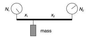
The scale readings tells us the normal or reaction force at each end of the bar. The condition of no translation in the y-direction yields
